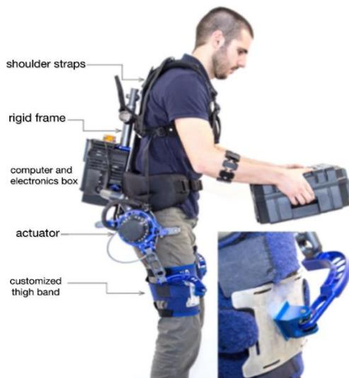
Fig. 14. The Mk2 prototype exoskeleton, as it is now worn by a user. This close-up of the customized thigh attachment, which consists of a stiff, bent metal plate attached to the thigh with a specially designed velcro strap, is shown on the bottom right. [48].
