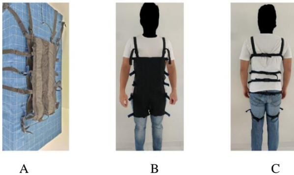
Fig.6. The designed of AireLevate exoskeleton (A) AireLevate. (B) The user's front view of the AireLevate device. (C) An image of the user's AireLevate's back [34].
