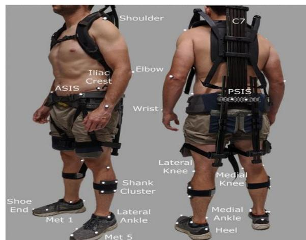
Fig. 18. Motion capture marker positioning. On the acromion process is where the shoulder marker is positioned. The lateral epicondyle of the humerus is where the elbow marker is positioned. The anterior and posterior superior iliac spines are referred to as ASIS and PSIS, respectively. Every marker is positioned on the subject's left and right sides. [54].
