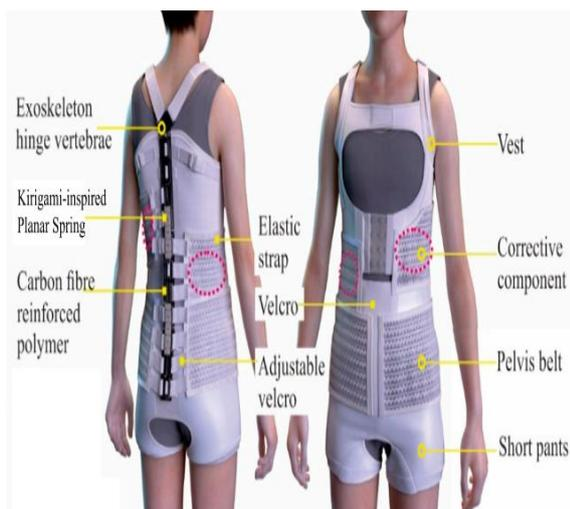
Fig.9. The exoskeleton hinge vertebrae's general design [36].
