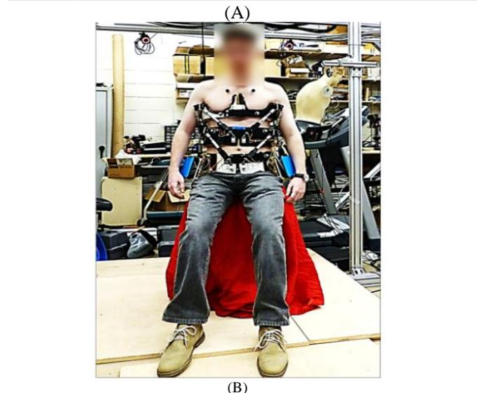
Fig.20. (A) RoSE uses a double parallel-actuated platform construction that incorporates sensors, motors, batteries, microcontrollers, and integrated electronics (B) Illustrative image of wearing the exoskeleton [56].
