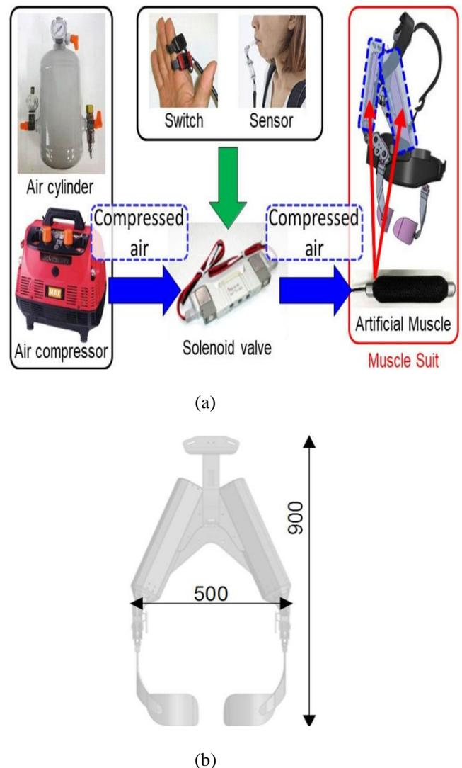
Fig.8. (a) Hardware components used to operate the muscle suit (b) The Muscle Suit CAD model's dimensions [6].
