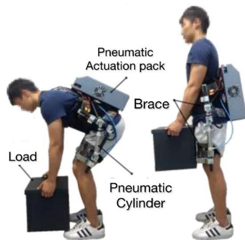
Fig.12. An overview is given by the pneumatic back support system for a portable exoskeleton. The microcompressor that is part of a pneumatic actuation pack allows the system to run on a pneumatic cylinder and makes it completely portable [46].
