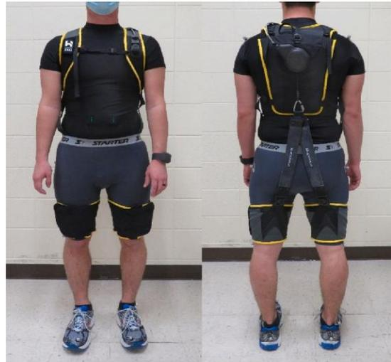
Fig. 2. Front and back images of a participant wearing the Apex (HeroWear, Nashville, USA). The exosuit is made up of two thigh sleeves, an upperbody portion that resembles a backpack, and two elastic bands that attach the upperbody portion to the thigh sleeves on the back. The study's sensors, such as the heart rate bracelet, optical tracking markers on the shoulders, and wireless electromyography sensors worn beneath the shirt, are also being worn by the participant.[28].
