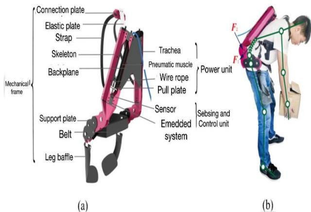
Fig.19. A power unit in the backpack, a sensing and control unit to regulate the power unit's efficacy, and a mechanical frame that distributes stresses to the shoulders and hips make up the wearable power assist device (a). When a person bends to lift large objects, the mechanical skeleton model uses a wearable power assist device (b) [55].
