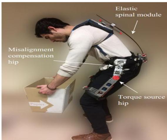
Fig.16. To relieve the lower back's burden, the SPEXOR passive back support exoskeleton combines torque generators with elastic beams (MACCEPA). In order to minimize discomfort and relative movement, misalignment compensation mechanisms are engaged at the hip and the back. This text has been taken from "Passive Back Support Exoskeleton Enhances Range of Motion with Flexible Beams." [51].
