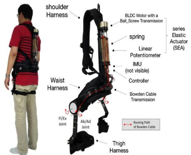
Fig.15. System architecture of our lifting assist device (LAD) prototype. (Color figure online) [50].
