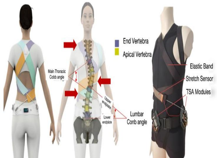
Fig.10. Conceptual design and prototype of a soft active brace [40].
