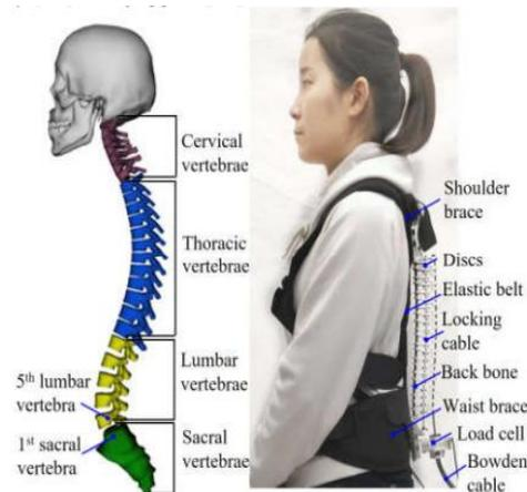
Fig.5. A tethered activation platform, wearable structure (shoulder and waist bracing), and a continuum mechanism make up the spine-inspired back exoskeleton. The spine-inspired soft exoskeleton is a unique design. This is a hyper-redundant, constantly bending continuum mechanism. The under-actuation robot provides assistance while adhering to the human spine's anatomical structure. The structure of the human spine does not impose any constraints on the natural move [8].
