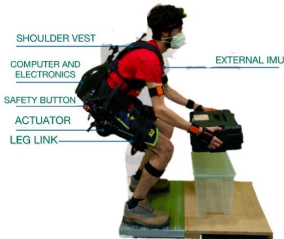
Fig.11. The experimental configuration involves a participant using the XoTrunk exoskeleton to perform tasks such as lifting and lowering a box. The shoulder vest front is where the IMU for acquiring linear acceleration is attached (at the sternum) [45].
